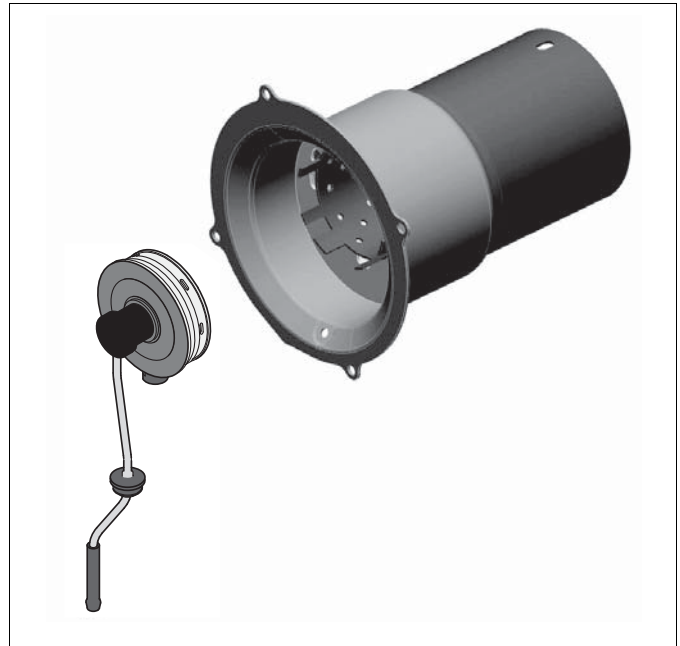
Fig. 206 Evaporator mount (petrol) and combustion pipe
